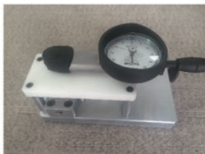
Screw head torque test 螺丝扭矩测量
